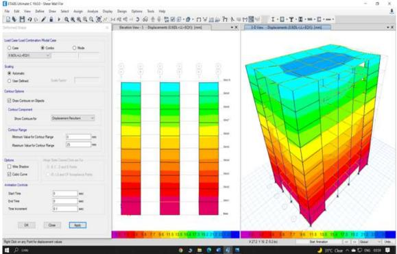
Contour Range = 0-25mm. Maximum Displacement =21 mm at top floor toward Center. **Deformed Shape Due to Load Combination 1.2(DL+LL+EQX)** Contour Range = 0-25mm. Maximum Displacement =22 mm at top floor toward Center.
