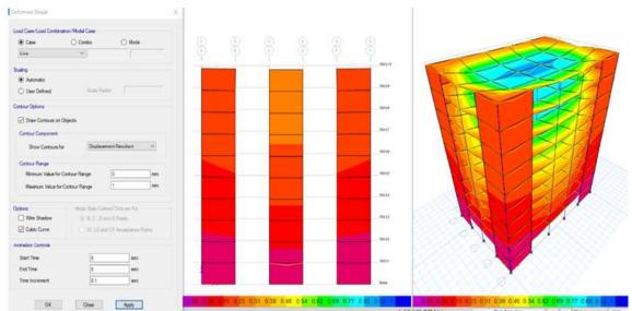
Contour Range 0-1 mm. As we can see maximum displacement is around center of the structure which is around 1mm.
