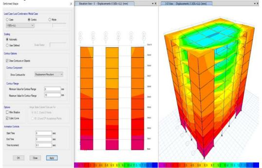
Contour Range = 0-15mm. Maximum Displacement = 13-14 mm at top floor toward Center.
