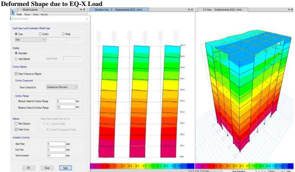
Contour Range 0-18mm. Maximum Displacement = 16 to 17mm at top floor toward Right.
