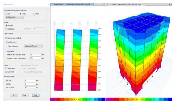
**Deformed Shape Due to Load Combination 0.9(DL+LL+EQY)**
