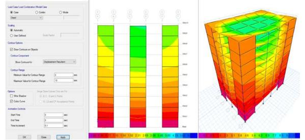
Contour Range 0 - 10 mm. As we can see maximum displacement is around center of the structure which is around 7mm.
